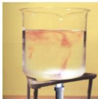
Figure 9.4: Crystals of potassium permanganate are used to show the movement of water on heating.
