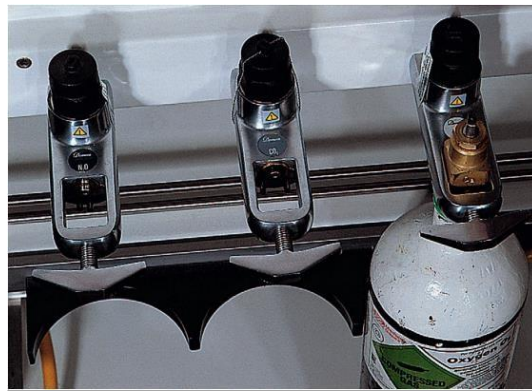
FIGURE 7-0 (A) Pin-index system. Note the different configuration for each gas. (B) Anesthetic machine cylinder yokes.
