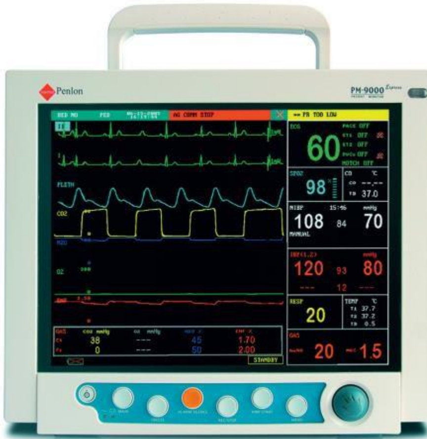
Fig. 11.17 The Penlon PM9000 Express which measures end-tidal CO 2 , oximetry and inhalational agent concentration using a side-stream method.
