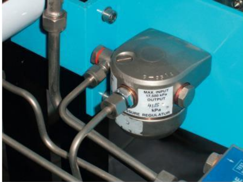
Fig. 8.8 Cylinder pressure regulator (the machine's tray has been removed)
