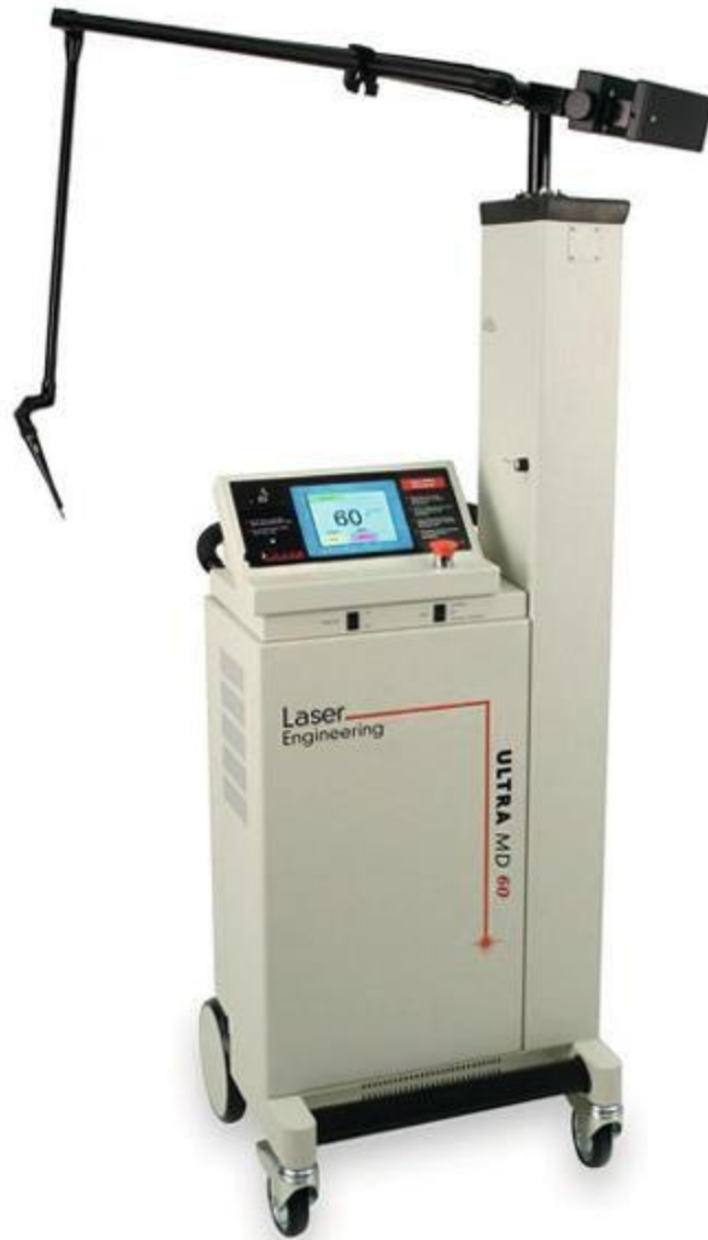
FIGURE 5.6. A typical CO2 laser showing the articulated arm with mirrors located at each joint that are necessary to reflect the laser beam down the arm. These mirrors are easily knocked out of alignment [arrangement], which can seriously affect laser function
