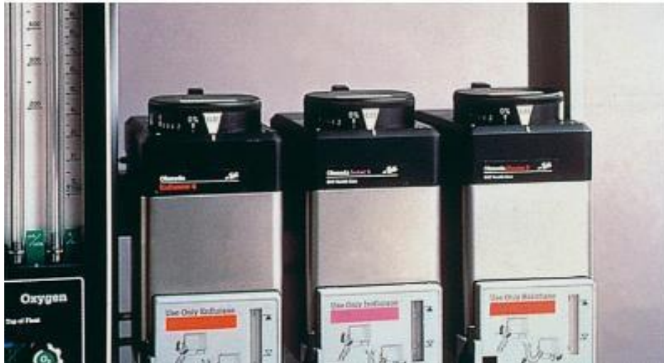
Fig. 8.17 Tec Mk 5 vaporizers mounted on the back bar of an Anesthetic machine.
