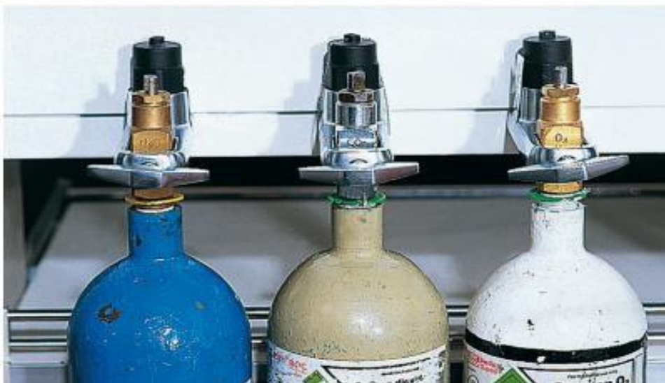
Fig. 8.7 Cylinder pressure regulators (black domes) positioned above the cylinder yokes in the Datex-Ohmeda Flexima Anesthetic machine
