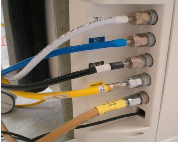
FIGURE 7-7 Color-coded hoses with NIST fittings attached to an anesthetic machine.
