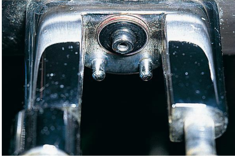
FIGURE 7-2 (A) A Bodok Seal. (B) A Cylinder yoke and Pin-index system. Note that a Bodok seal is in position.
