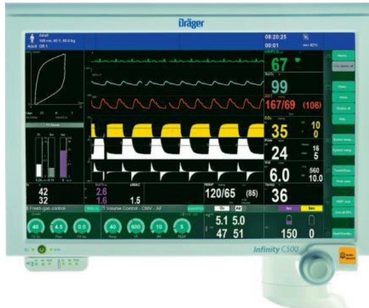
Fig. 11.3 Colour-coded values and waveforms displayed on the Zeus Dräger monitor. (Courtesy of Dräger.)
