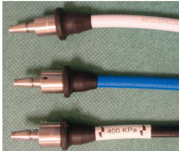
FIGURE 7-5 Gas probes for oxygen (top), nitrous oxide (middle) and air (bottom). Note the locking groove on the probe to ensure connectivity.
