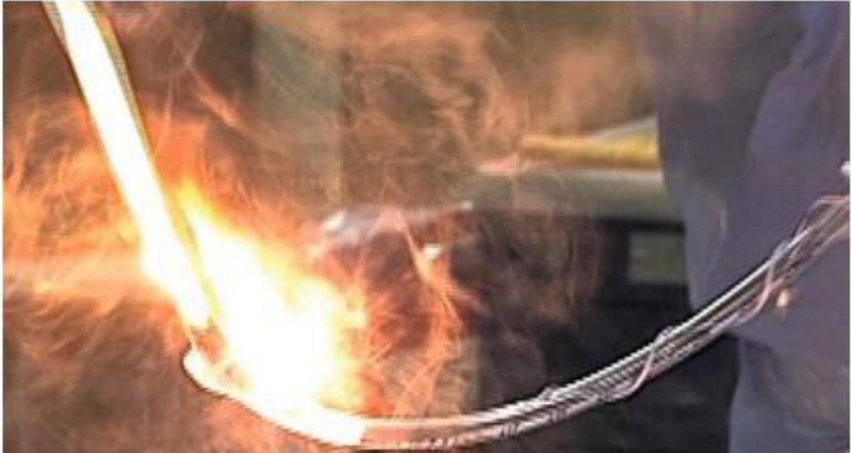
FIGURE 4.2. Ignition of an ETT results in a fire that resembles a blowtorch. What cannot be appreciated from the photo are the acrid products of combustion, which can significantly impair respiratory function.
