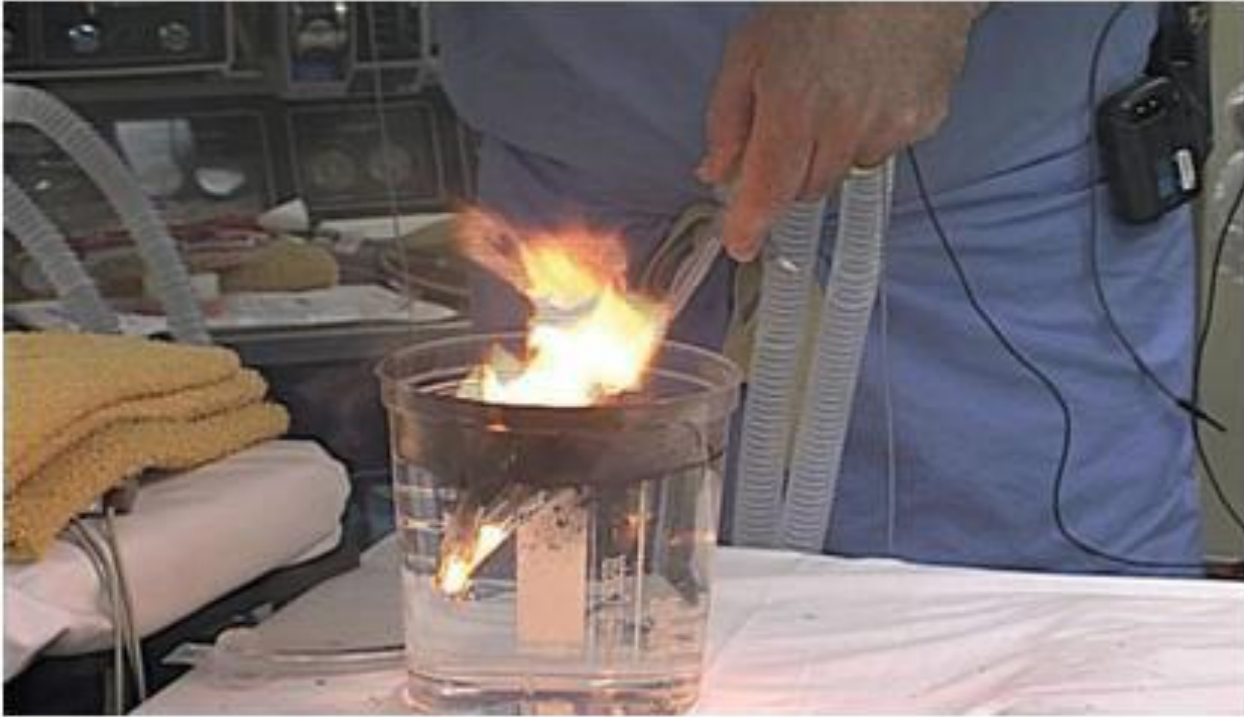
FIGURE 4.3. An ETT on fire continues to burn, despite being submerged underwater. Note the fire present within the portion of the tube that is below the surface of the water.
