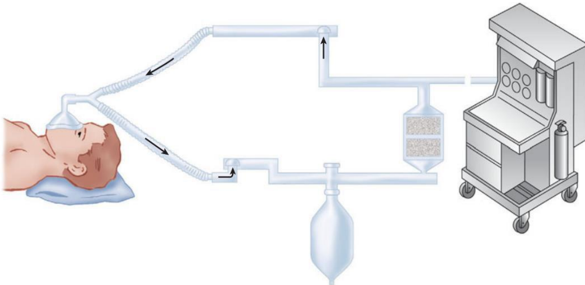
Figure. 9-1. The relationship between patient breathing circuit and anesthesia machine
