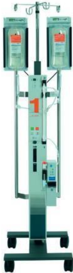
Fig. Smiths Medical Level 1 H 1200 fast fluid warmer with an integrated air detector.
