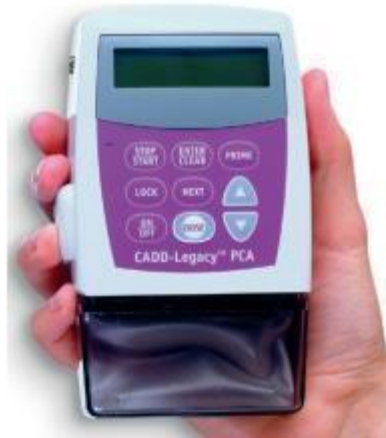
Fig. The CADD Legacy portable PCA.
