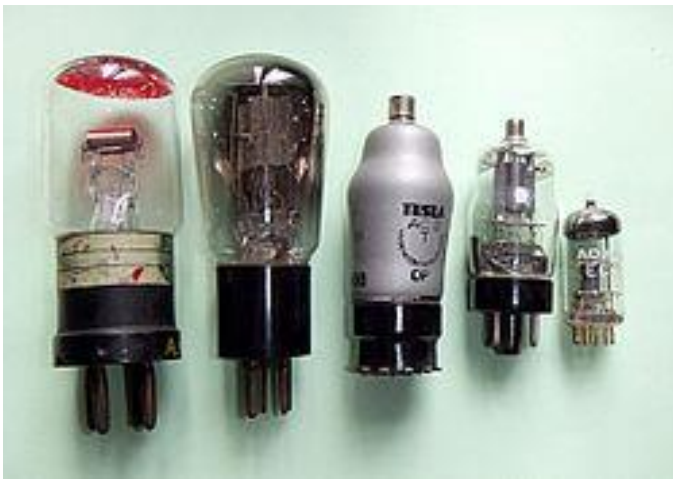
Examples of low power triodes from 1918 (left) to miniature tubes of the 1960s (right)
