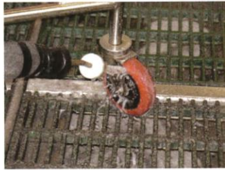
Example of a spray nozzle system for cleaning mobile equipment and cart wheels.
