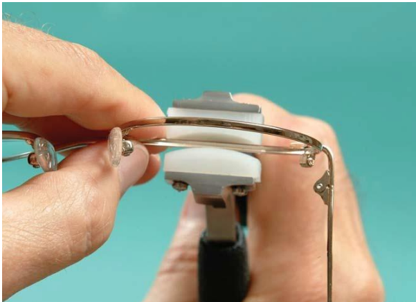
Figure 7-15. To increase the curve of the eyewire of a metal frame, position the eyewire forming pliers as shown in the photo and gently squeeze, repositioning the pliers as necessary.
