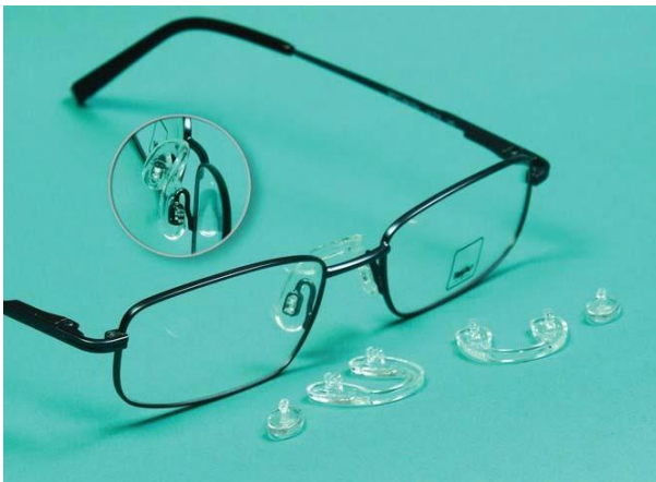
Figure 10-44. A strap bridge replaces two adjustable pads. It distributes frame weight over both the traditional nosepad areas and across the crest of the nose. The flexibility of the material allows both pads to still be adjusted separately.
