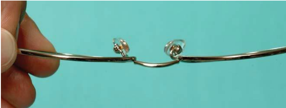
Figure 9-41. In this photo, the pad angles are basically symmetrical, but the pads themselves are moved too far to one side. This defect as shown from above will cause the frame to sit too far to the wearer's left, as was shown in the previous figure.
