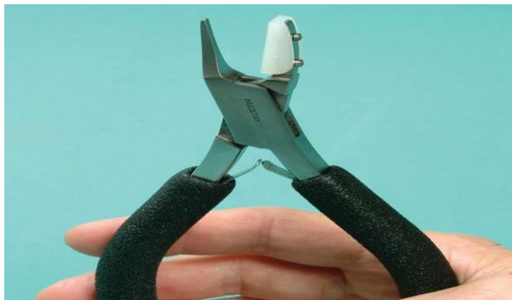
Figure 8-18. Half-padded pliers hold the frame securely. The nylon-padded jaw prevents the frame from being marred by that jaw of the pliers. The unpadded jaw may be flat or rounded.
