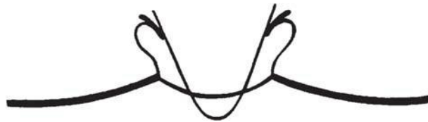
Figure 9-32. This illustration, viewed from the top in cross section, shows a pad splay angle too great for the nose. The splay angle of the pads must be decreased.
