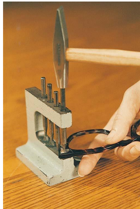
Figure 10-52. One method for removing rivets is tapping the old rivet out with a hammer and punch.
