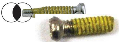
Figure 10-9. This type of self-locking replacement screw has an epoxy type of coating on the threads that keeps the screw from backing out. It is removable and can be used again. As would be expected, each time it is taken out and replaced, it loses some of its adhesive characteristics.
