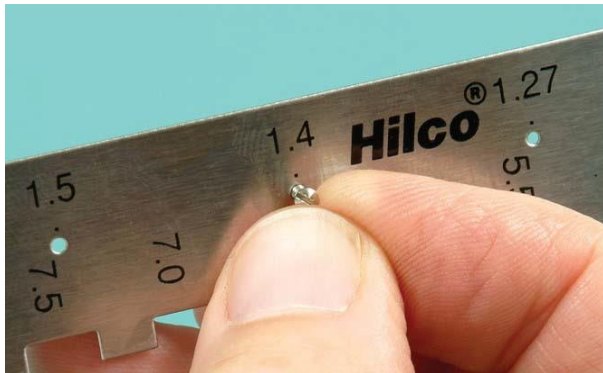
Figure 10-19. To find the diameter of the screw, slip the screw through each hole until a match is found. Incidentally, this 1.4 mm diameter is the most commonly used diameter for optical screws.
