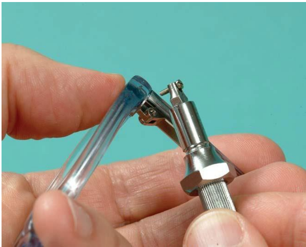
Figure 10-5. The screw-holding tool places the screw in hard-to-reach places where fingers cannot always go.
