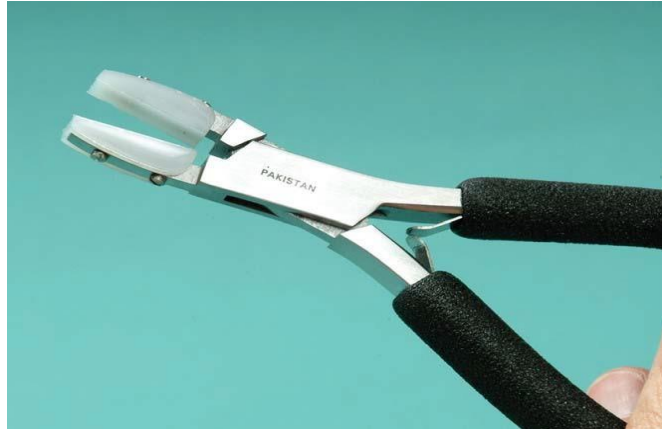
Figure 8-48. Double-padded pliers help to prevent marks on the frame during frame adjustment.
