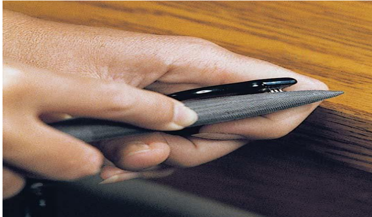
Figure 8-22. Even though a specially designed bench brace is the method of choice, a frame may be successfully held for filing by bracing one knuckle over the edge of a table.
