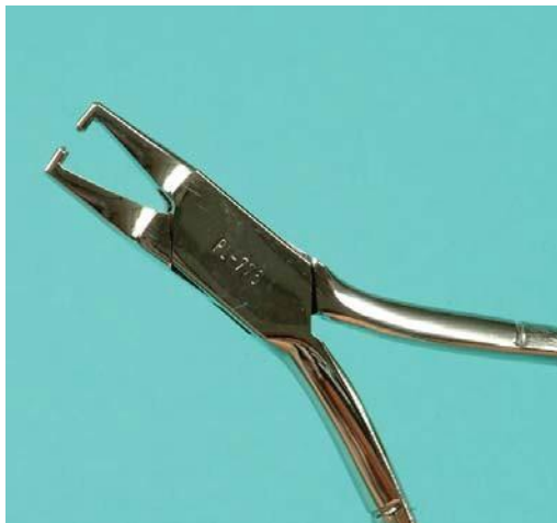
Figure 7-15. To increase the curve of the eyewire of a metal frame, position the eyewire forming pliers as shown in the photo and gently squeeze, repositioning the pliers as necessary.
