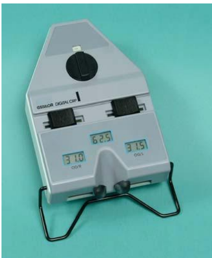
Figure 3-6. The digital version of Essilor’s pupillometer displays monocular PDs for the right and left eyes, as well as the binocular PD. It can be set to measure distance or near PDs.
