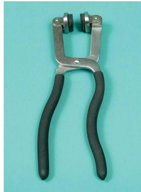
Figure 7-8. Many different types of lens twisting pliers are available. There are two important variations in these pliers.
