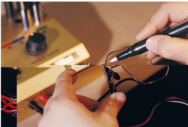
Figure 10-88. Frames are buffed after soldering to remove foreign matter and discoloration. The tiny rag wheel is mounted on a Dremel tool or a hanging motor drill.
