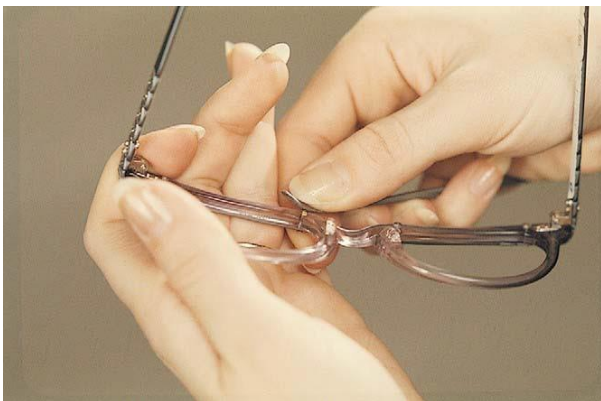
Figure 10-80. The rough end of the clipped-off screw is filed smooth with a riffler file. Although it may appear easier, inserting the lens before attaching the plaques may stretch the upper part of the eyewire. As a result, the predrilled holes in the chassis separate slightly so that the screws that pass through the plaque no longer pass through the holes in the chassis. In this event, drill one or more new holes to reattach the plaque.
