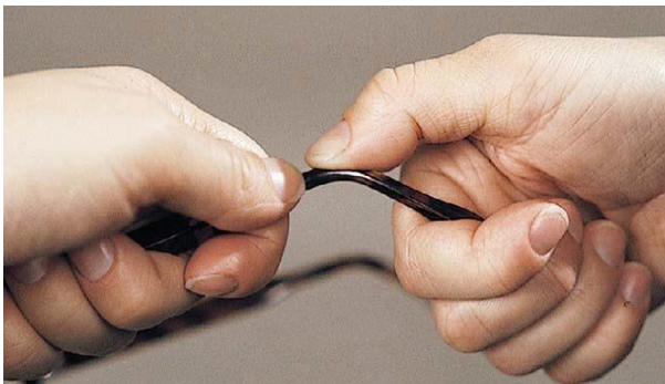
Figure 9-18. Straightening the temple to move the bend to a new location may be done as shown. If the bend is to be moved forward, it may also be done by first placing a new bend at the desired location; then removing the old bend.
