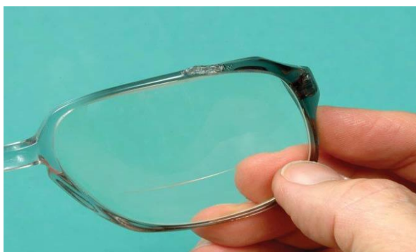
Figure 8-1. An example of a frame that has been overheated, resulting in bubbling of the plastic on the upper rim.
