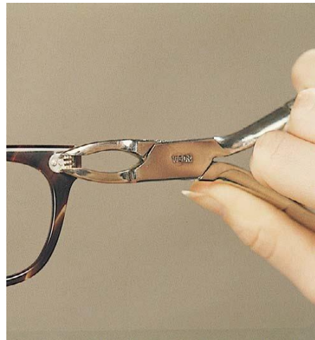
Figure 10-17. Now the temple will fit into the frame front, and all of the barrels will line up. The screw should now go in as if the frame had a normal temple barrel configuration.
