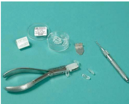
Figure 9-64. Silicone nose pads mounted onto plastic frames with adhesive or with small drilled holes will not only reduce slippage, but also slightly narrow the effective
