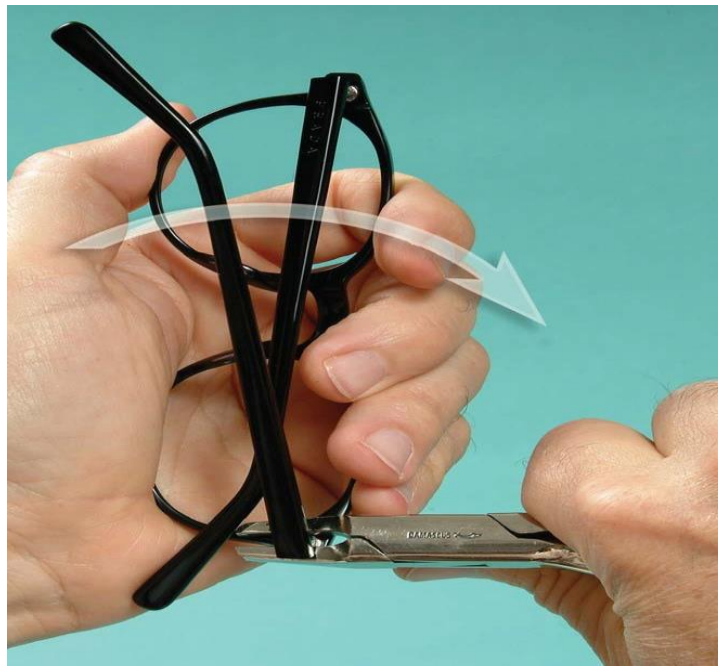
Figure 8-35. With the temple folded, finger-piece pliers are held parallel to the endpiece hinge screw so that the hinge is grasped on both sides.
