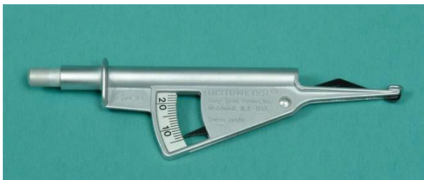
Figure 5-13. A distometer measures the distance from the back surface of the lens to the front surface of the eye.
