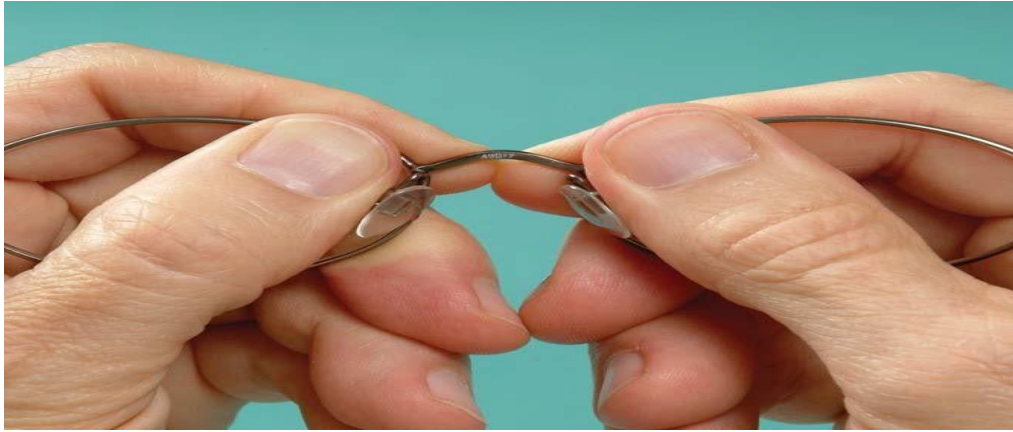
Figure 8-38. This is how the hands are held to either change the face form of a metal frame or to remove X-ing. Care must be taken because undue stress at the lens/eyewire area may result in chipping of the lens edge.
