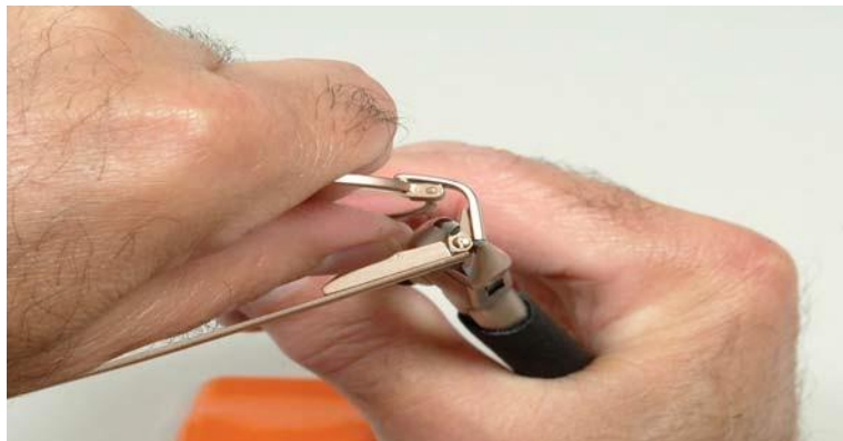
Figure 8-45. Use the hand to grasp the frame front firmly at the endpiece. Decrease temple spread with the pliers. If there is risk of chipping the lens, remove the lens first.
