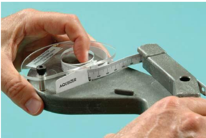
Figure 6-24. To measure the circumference of a lens, place the lens in the gauge front-side-up. Close the tape around the lens and read the circumference directly
