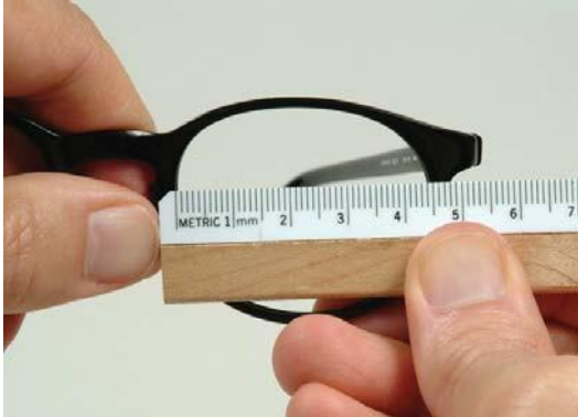
Figure 2-3. To measure the horizontal dimension of a frame, the measurement begins at the inside of the groove on one side and extends across the lens opening to the farthest part of the groove on the other. We cannot see the inside of the groove when looking from the front. This means we can estimate where it will be and hold the ruler so that the zero point is at the position of the left-hand side of the groove. Then we need to read the ruler at the position where the groove will be on the right. If the opening itself is measured, then about ½ mm per side needs to be added to the measure to allow for the depth of the groove. This may vary somewhat, depending upon the depth of the groove.
