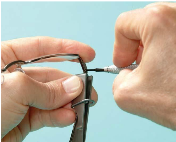
Figure 10-17. Now the temple will fit into the frame front, and all of the barrels will line up. The screw should now go in as if the frame had a normal temple barrel configuration.
