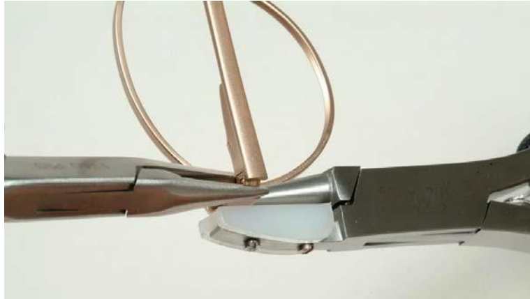
Figure 8-46. The risk of lens chipping can be reduced by using holding pliers while reducing temple spread.
