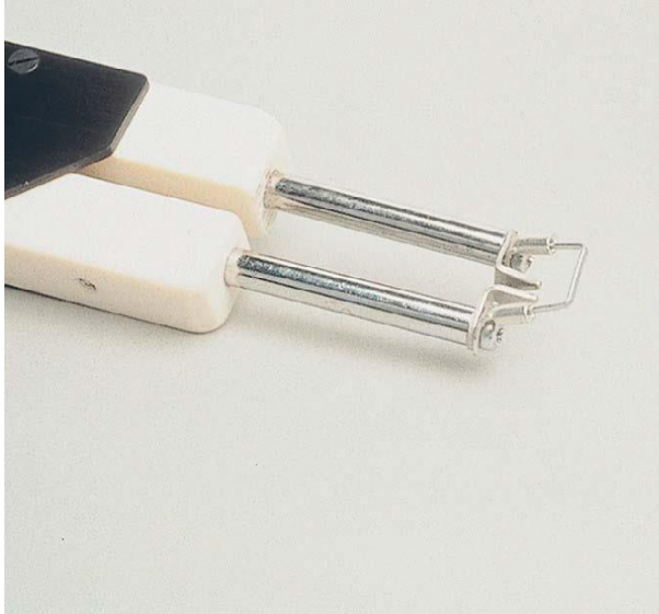
Figure 10-64. The Hot Fingers repair unit can be used to fix a broken bridge with a commercial grade \frac{1}{4} -inch staple. The staple is grasped securely with the staple adapter. (Courtesy Hilco, Plainville, Mass.)
