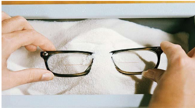
Figure 8-2. To heat the bridge area, first form the salt into a centrally located peak running across the pan, then draw the bridge through the peak of the salt mound.
