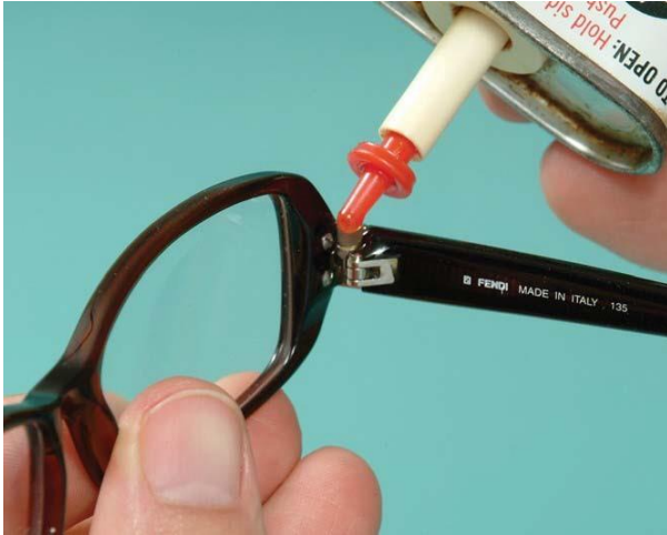
Figure 10-24. Penetrating oil, such as “Liquid Wrench” auto- motive penetrating oil, helps cut corrosion and loosen stuck screws.
