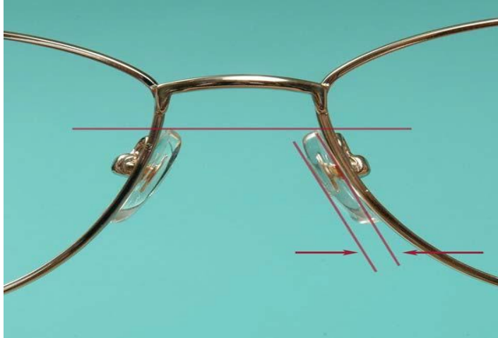
Figure 8-59. An estimated ideal position is that in which the faces of the pads appear approximately 1 mm closer to the nose than the eyewire itself. Both pads should also be at the same height, as shown by the horizontal red line.
