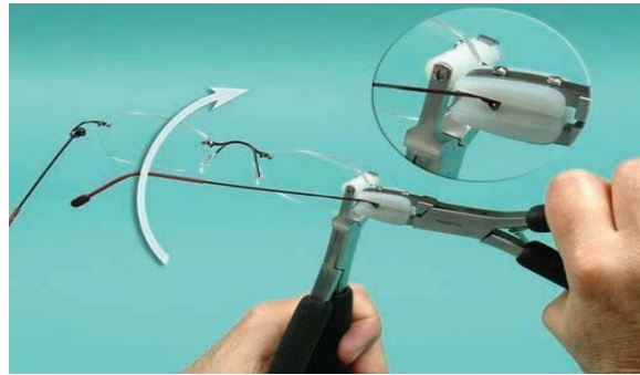
Figure 8-75. A very popular variation on changing the pantoscopic angle uses endpiece angling pliers to angle the temple.
