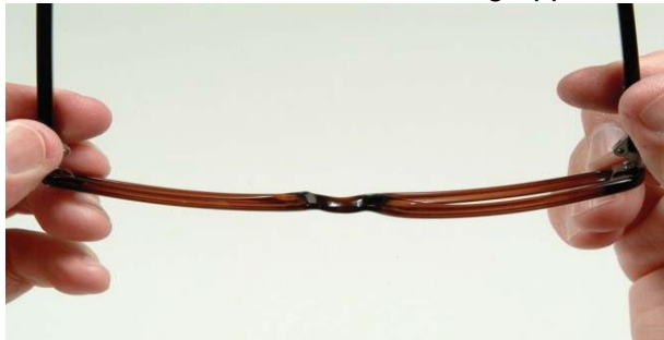
Figure 8-11. This is how a frame with X-ing appears when viewed from below.
