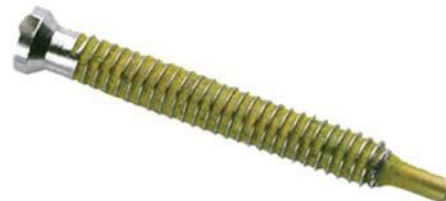
Figure 10-37. A self-tapping screw cuts its own threading. After the screw is fully in place, the excess is broken off with pliers. (Courtesy Hilco, Plainville, Mass.)
