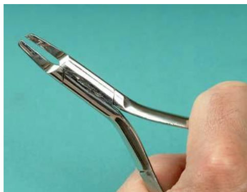
Figure 8-34. Finger-piece pliers were originally designed for adjusting the old
