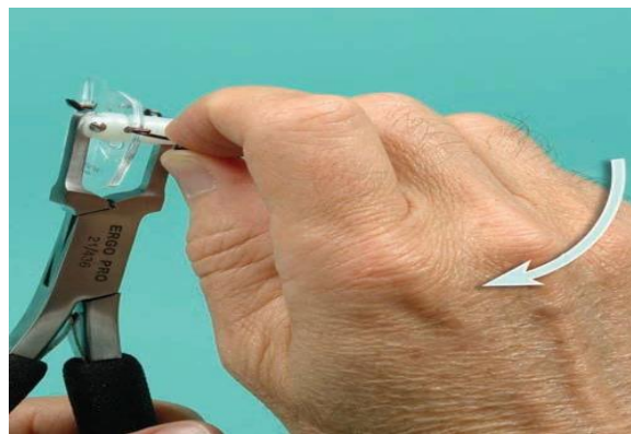
Figure 8-76. A quick alternative for changing the temple's pantoscopic angle uses rimless bracing pliers to hold and makes the bend with the free hand.
