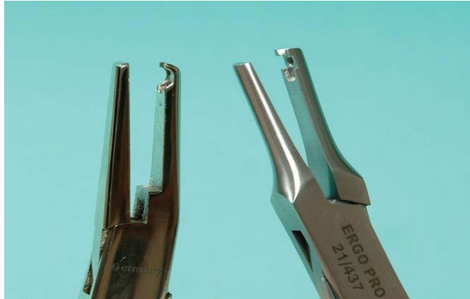
Figure 8-57. The type of pad-adjusting pliers used will depend on the type of pad on the frame.
