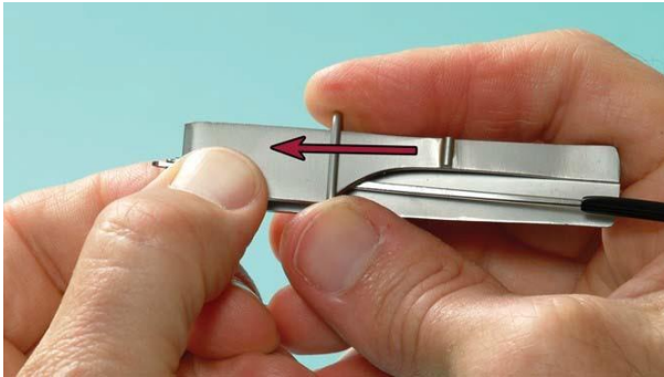
Figure 10-16. While squeezing the spring hinge alignment tool to keep the barrel extended, slip the slide forward so that the alignment tool will not open.
