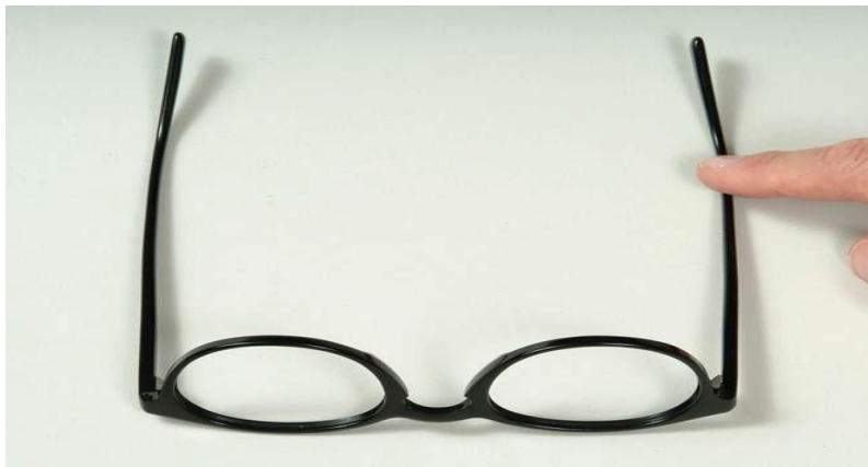
Figure 8-25. Testing for parallelism using the flat surface touch test
