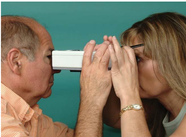
Figure 3-7. To use a pupillometer, the subject (on the right) holds the pupillometer so that the pads rest on the nose in the manner of normal eyeglasses. The dispenser views the subject's eyes through the instrument.
