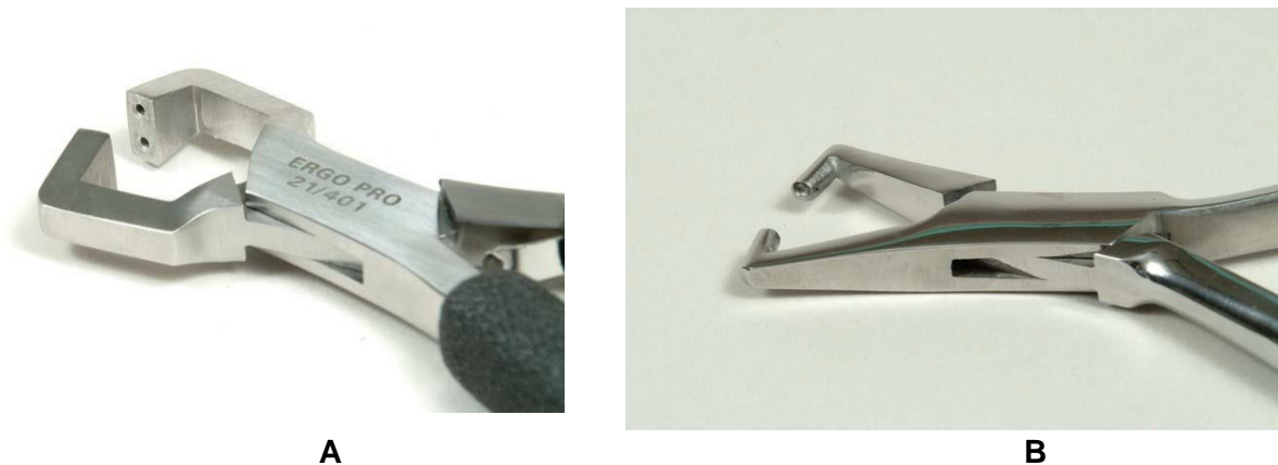
Figure 8-28. Angling pliers. Traditional angling pliers are shown in (A) . Note the indentations on the inside of the jaws used to grip the screw. Since these pliers are a bit bulky and sometimes difficult to get into hard-to-reach areas, a modified, a narrower version is shown in (B) .
