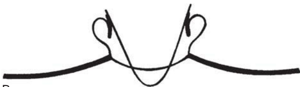
Figure 9-33. In A the splay angle of the pads needs to be increased. The back edges of the pads will cut into the flesh of the nose unless
