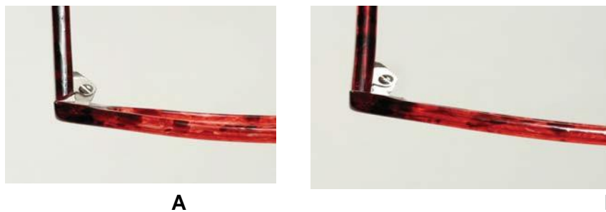
Figure 8-24. Viewed from the top, the frame in (A) shows how temple and front should abut. The improperly filed temple in (B) will not hold alignment. Because so much force is on such a small area, within a short period of time the plastic
