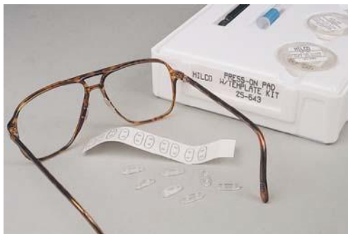
Figure 10-67. Here are the necessary items for mounting press-on build-up pads to a plastic frame. All items are available as a kit. Pads are available in either acetate (regular hard plastic) or silicone (pliable, slip-resistant material). (Courtesy Hilco, Plainville, Mass.)
