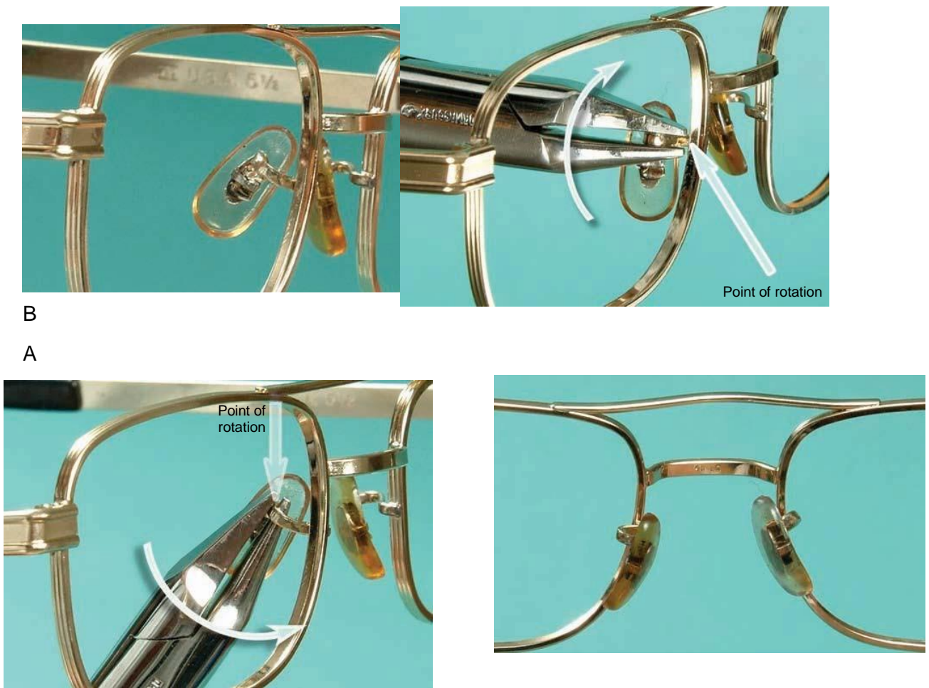
Figure 9-55. A , To raise the pads on frames with question mark pad arms, thin pliers are used to grasp the entire pad arm and bend it upward. This will lower the frame on the face. B , After the question mark type pad arm has been bent upward, the pad will be considerably higher, but has an incorrect vertical angle. The pad must be reangled. C , Reangling the pad to correct the vertical angle after having raised the question mark style pad arm is done by grasping the curl close to the pad. This can be done with square round (or thin-nosed) pliers as shown here. D , Note how much higher the pad on the right is than the pad on the left. When both pads are adjusted, the frame will sit considerably lower than previously.
