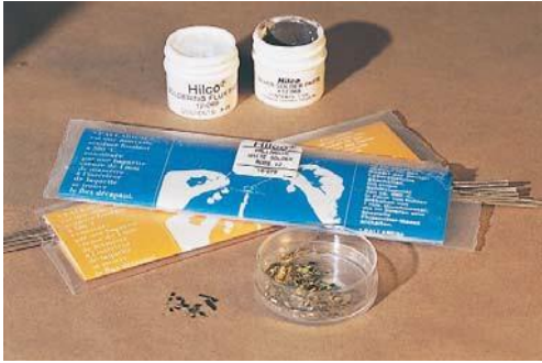
Figure 10-82. Solder comes in a variety of forms and must be used in conjunction with soldering flux . Flux is shown in the upper left-hand container. There is a silver solder paste that combines both solder and flux. This is seen in the upper right-hand container. Solder is available in rod form , as pictured in the plastic envelope in the center of the photo. The chip form of solder, at the bottom of the photo, is particularly useful for electric soldering. (Courtesy Hilco, Plainville, Mass.) to the laboratory or elsewhere for repairs, soldering sometimes provides a definite service to the wearer. It also sets the office apart from others and provides another unique service.
