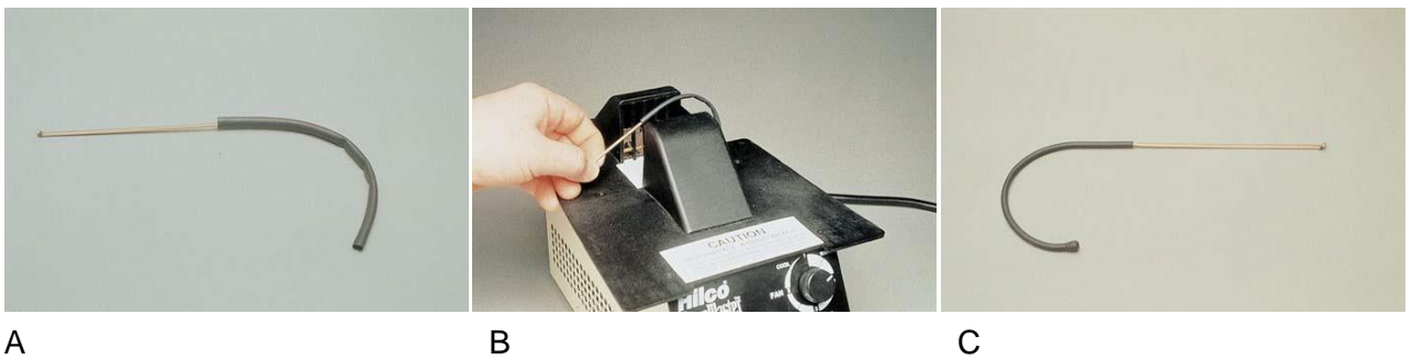
Figure 10-45. It is possible to cover the end of a cable temple with heat-shrink cable tip covers. Find the correct diameter, cut to length, and slip over the end of the cable temple, as shown in A . Heat using a frame warmer on the highest setting, as shown in B . Heat-shrink cable tips tighten up snugly, as seen on the temple shown in C . (Courtesy Hilco, Plainville, Mass.)
