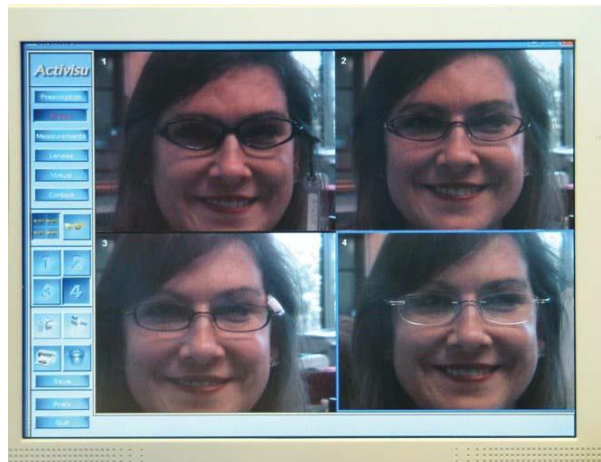
Figure 4-24. Here the image system permits side-by-side comparisons of different frames on the same screen.
