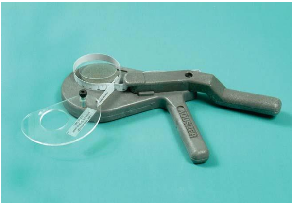
Figure 6-23. A circumference gauge is used to find the circumference of an edged lens.
