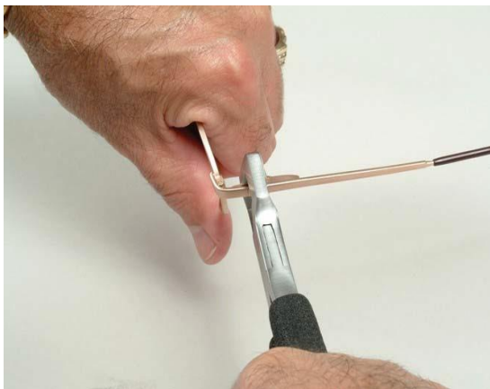
Figure 8-50. When the endpiece is too small, the pantoscopic angle can be changed without holding pliers. If the frame does not have enough flexibility, the lens may be removed first.
