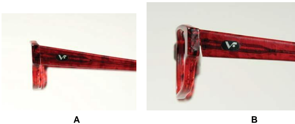
Figure 8-23. The frame pictured in (A) shows the proper abutment between temple and frame front, whereas the frame in (B) is the result of uneven or hurried filings.
