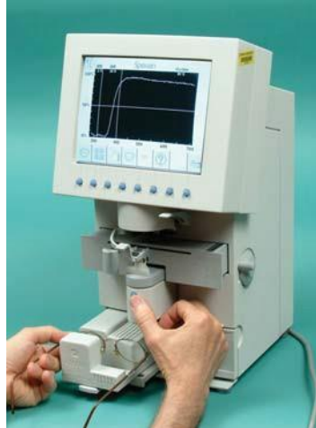
Figure 6-40. Some models of the Humphrey Lens Analyzer autolensmeter will allow the transmission of a lens to be measured. The readout is in the form of a transmission curve.
