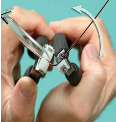
Figure 8-71. A , To increase or decrease the temple spread for a rimless mounting, grasp the temporal point of attachment of the lens with rimless bracing pliers. Then grip the endpiece with half-padded pliers from above and bend the endpiece either outward or inward. B , Some may prefer to grip the endpiece area from below with both pliers to bend the endpiece in or out. C , Hold the frame front steady with rimless bracing pliers ( left ) and rotate the half-padded pliers to bend the endpiece, bringing the temple inward or outward. D , Tri-angling pliers may be used to increase or decrease temple spread on certain rimless frames without putting stress on the lenses.
