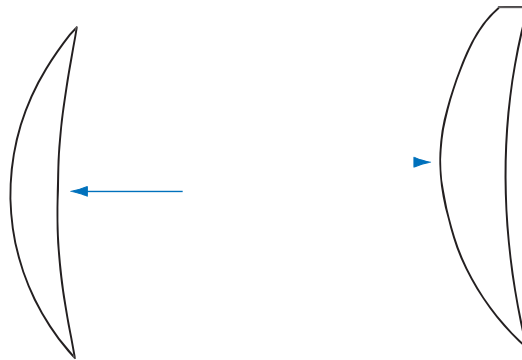
Figure 5-12. These two high plus lenses have the same refractive power. The lens on the left has the optical center half way between the top and the bottom. The lens on the right has the optical center too high for a lens of this power. As a result, the upper edge is excessively thick. and choose one that will place the eyes higher in the frame, (b) reduce the pantoscopic tilt, or (c) just not lower the MRP
