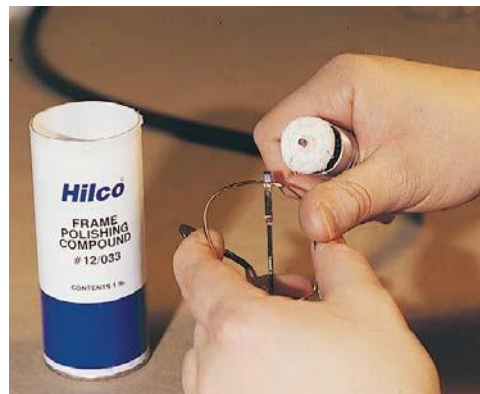
Figure 10-88. Frames are buffed after soldering to remove foreign matter and discoloration. The tiny rag wheel is mounted on a Dremel tool or a hanging motor drill.
