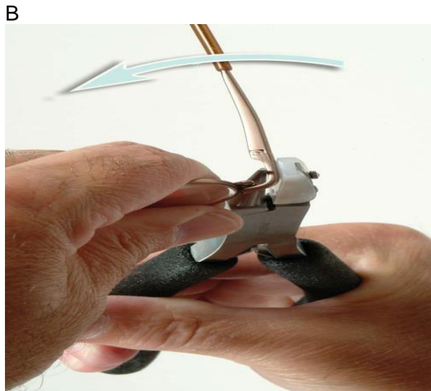
Figure 8-44. If the temples are spread too far apart, a pair of half-padded pliers may serve as bending pliers and grip the outside of the endpiece. A , Side view. B , Top view.
