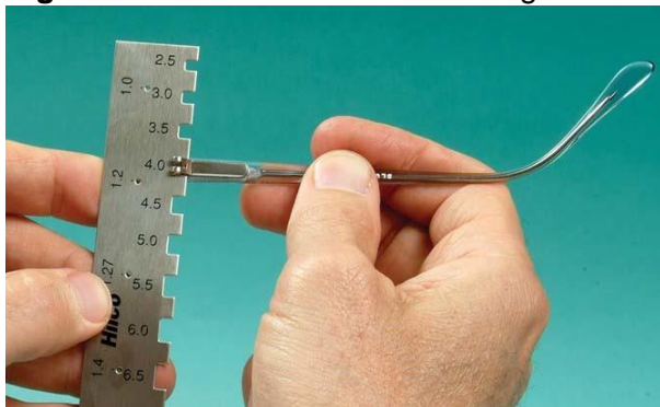
Figure 10-20. To find the screw length for a missing screw, measure the depth of the
